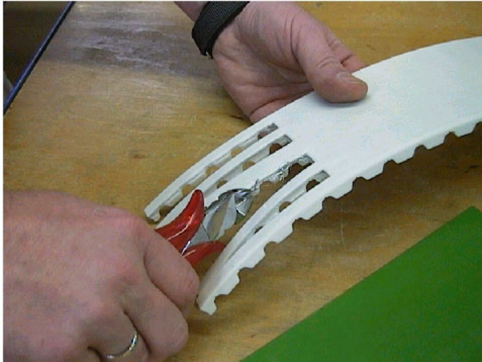
Illustration 3: Remove stray wires in the die-cut area of the timing belt.
