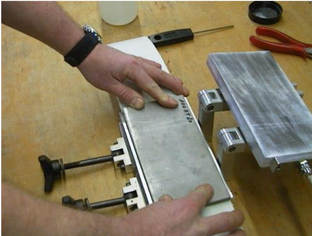
Illustration 11 : Position the pressure plate over the weld area of the timing belt.
