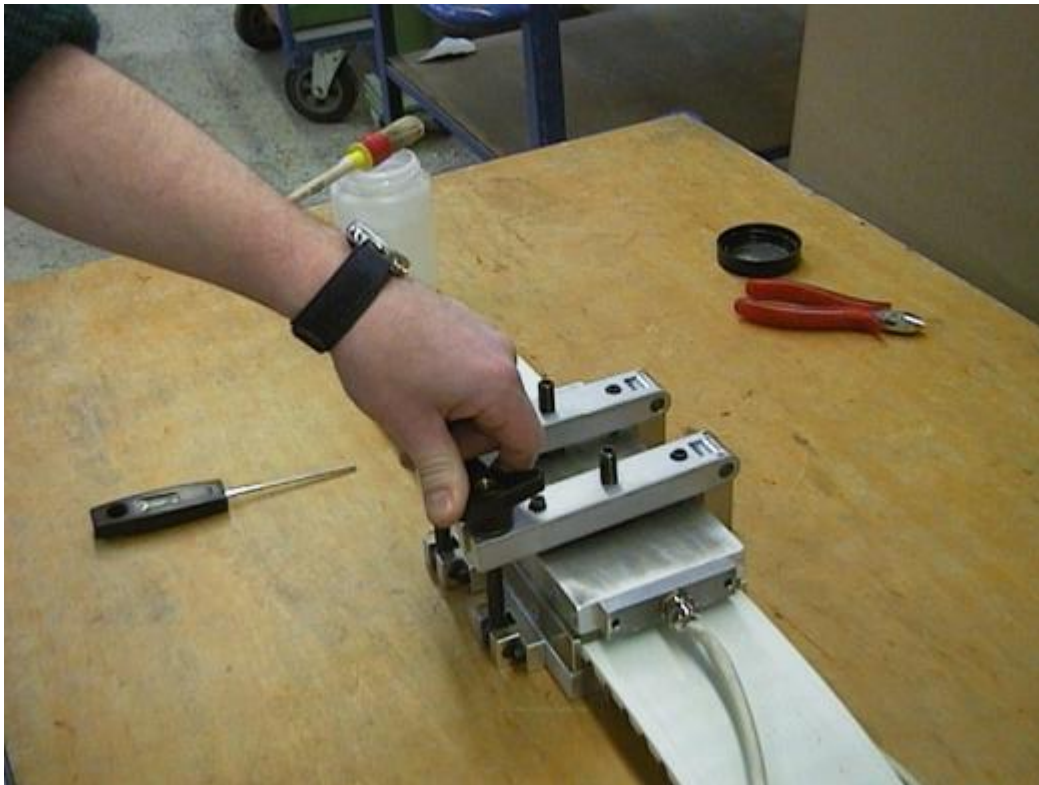
Illustration 14 : Tighten top plate with wing nuts
